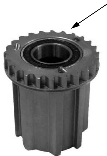
12 Tooth 3-Pin Style 15mm cassette body.
