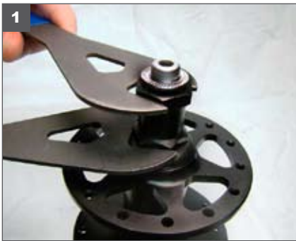
1. Using two 19mm cone wrenches, hold the bottom adjusting nut in place and loosen the top lock nut.
