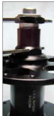
1. Using two 19mm cone wrenches, hold the bottom adjusting nut in place and loosen the top lock nut.
