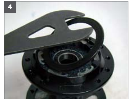
4. Remove large black pawl seal from the hub shell (if your hub has one).
