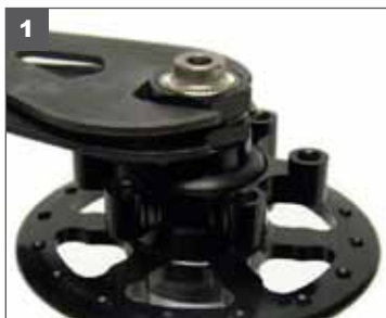
1. Using two 19mm cone wrenches, loosen the lock and adjusting nut.
