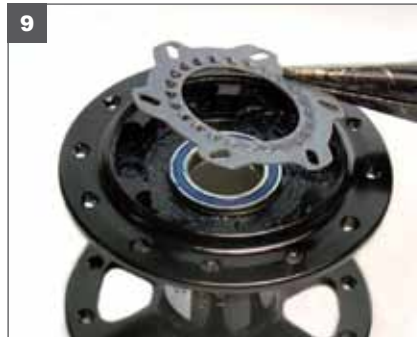
9. With a thin layer of clean grease coating the hub shell, install the cam plate. Refer to the picture for the correct orientation. Do not put the cam plate in upside down.
