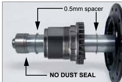
SRAM XD Axle Assembly.
