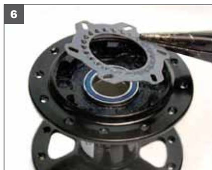
6. Remove cam plate.
