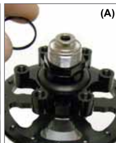
A. Some, but not all, hubs have a 1.5mm axle spacer.
