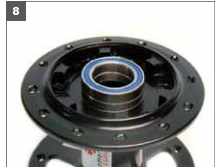
8. Bearing Installation: Position a new bearing onto the hub shell. Place old bearing on top of new bearing.
