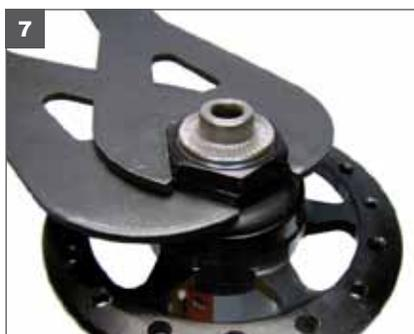
7. Thread the 19mm adjusting nut with dust seal attached onto the 9mm quick release axle and tighten with a wrench. Tighten the adjusting nut until there is no play and back off one quarter rotation.
