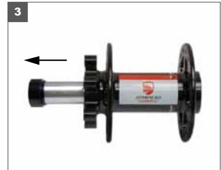
3. Push the 15mm thru axle to the disc side, and pull the axle from the hub.
