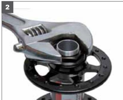
2. Using a 22mm wrench, turn counter clockwise to loosen and remove the adjusting nut.
