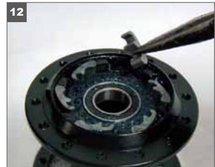
12. With a thin layer of clean grease coating the top of the cam plate, install all 6 pawls. Once completed, the pawls should freely engage in unison with the cam plate.
