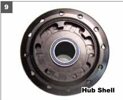
9. Clean out the hub shell for inspection and new grease.
