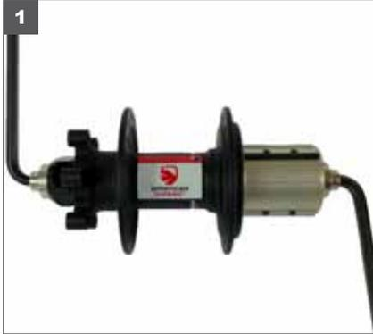
1. Insert a 5mm hex wrench into each end of the silver endcaps (where quick release goes through, one on each side).
