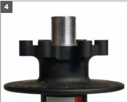
4. Once the end cap and adjusting nut are removed, you are ready to open the hub.
