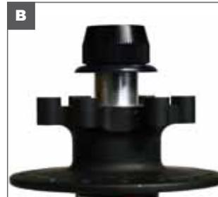
B. Tighten the adjusting nut with dust seal until snug against the bearing. The O-ring inside the adjusting nut provides drag to hold the bearing adjustment.
