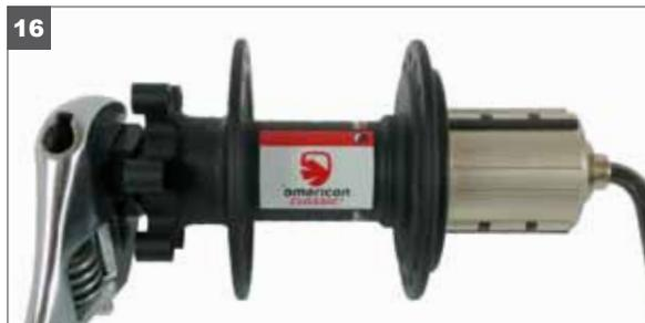
16. Insert the 5mm hex wrench into the cassette side end cap. Holding the hex wrench in place, the hex adjusting nut can be used to adjust the play. The internal O-ring will hold it in place, no lock nut is required. This can be done with fingers or with an adjustable wrench.
