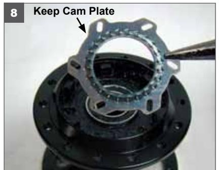
8. Remove cam plate. **IMPORTANT:** Keep cam plate for re-installation in Step 11.
