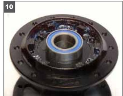
10. Bearing Installation: Position a new bearing onto the hub shell. Place old bearing on top of new bearing.
