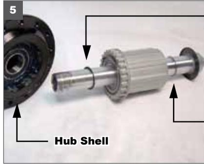
5. Separate the cassette body and axle from the hub shell by grabbing the body with your hand and pulling it out from the drive side.
