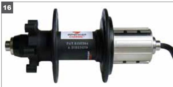
16. Insert the 5mm hex wrench into the cassette side end cap. Holding the hex wrench in place, the knurled adjuster can be used to adjust the play. The internal O-ring will hold it in place, no lock nut is required. This can be done with fingers or with pliers.
