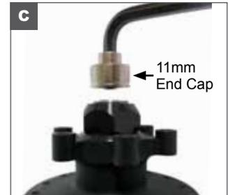
C. Keep 5mm hex wrench in drive side. Thread on the 11mm end cap with another 5mm hex wrench.
