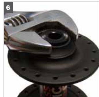
6. Install and adjust the remaining Terrain 9mm Thru Axle Quick Release cap. The threaded cap must be snug, not loose. Do Not overtighten.
