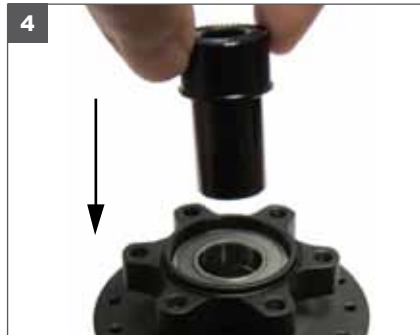
4. Slide the Terrain 9mm Thru Axle Quick Release adapter into the hub, resting the small lip on the inner race of the bearing.
