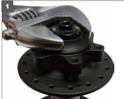
1. Using a 22mm wrench, turn counter clockwise to loosen and remove the large black threaded cap.
