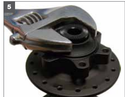
5. Place the large black threaded cap over the Terrain 9mm Thru Axle Quick Release cap and thread into the hubshell. This cap has no bearing adjustment and should be tightened down.
