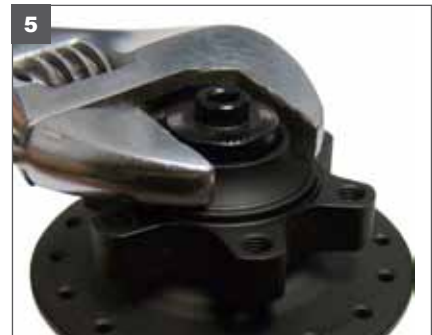
5. Place the large black threaded cap over the Terrain 9mm Quick Release cap and thread into the hubshell. This cap has no bearing adjustment and should be tightened down.
