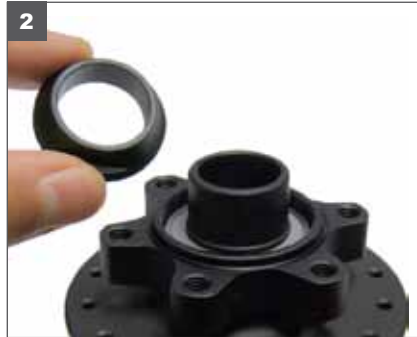
2. Remove large black threaded cap.
