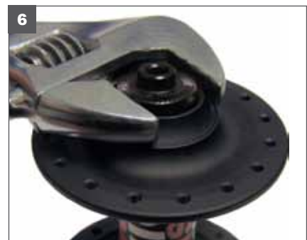
6. Install and adjust the remaining Terrain 9mm Quick Release cap on the non-disc side. The threaded cap must be snug, not loose. Do Not overtighten.
