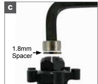
C. Keep 10mm hex wrench in drive side. Place the 1.8mm spacer on the axle and thread on the end cap using another 10mm hex wrench.
