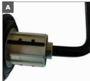
A. Insert 10mm hex wrench into drive side end cap. Keep the 10mm hex wrench in place.
