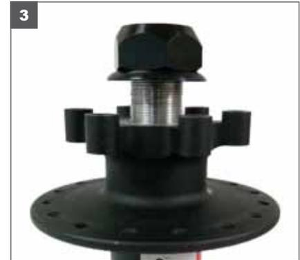
3. Keep the 5mm hex wrench in drive side (side with cassette) end cap to hold the axle in place and unthread the hex or knurled nut with dust seal.
