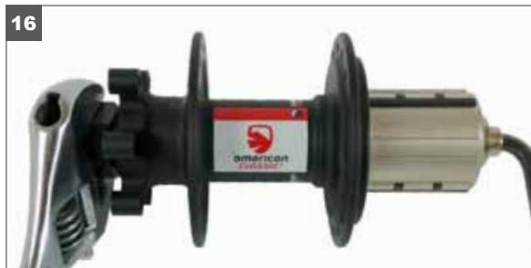
16. Insert the 10mm hex wrench into the cassette side end cap. Holding the hex wrench in place, the hex adjusting nut can be used to adjust the play. The internal O-ring will hold it in place, no lock nut is required. This can be done with fingers or an adjustable wrench.
