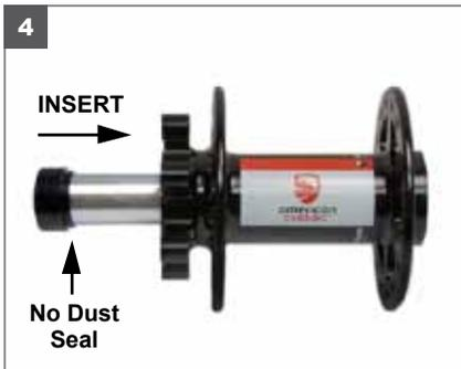
4. Insert the BOOST 15mm x 110mm thru axle from the disc side of the hub. Dust Seal is installed in Step 9.
