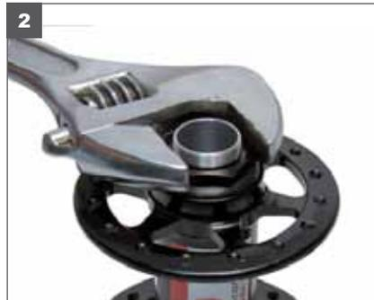
2. Using a 22mm wrench, turn counter clockwise to loosen and remove the 22mm Adjusting Nut.
