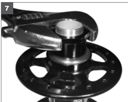
7. Thread the 22mm Adjusting Nut onto the end of the 10mm Spacer and tighten with a wrench. Tighten the adjusting nut until there is no play and back off one quarter rotation.
