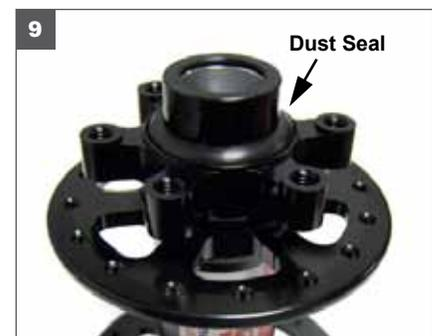
9. Finally slide the remaining dust seal over the end cap on the disc side.
