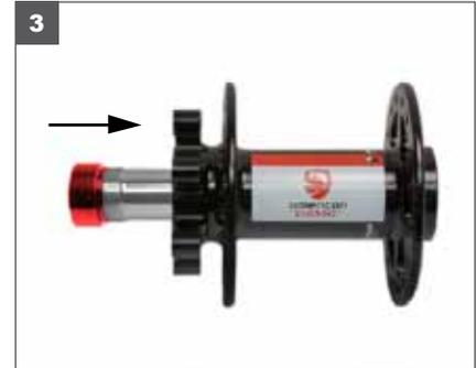
3. Insert the 12mm Thru Axle from the disc side of the hub.
