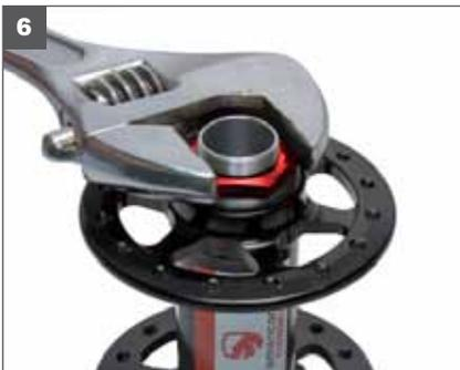
6. Thread the 22mm Adjusting Nut with dust seal attached onto the end of the 12mm Thru Axle and tighten with a wrench. Tighten the adjusting nut until there is no play and back off one quarter rotation.
