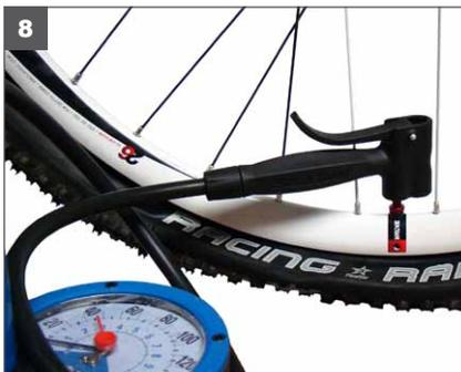
8. With the valve core installed, pump air back into the tire and seat the tire beads.
