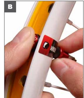
B. Firmly press valve base into rim with your thumb and finger to tighten knurled nut.
