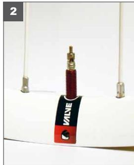
2. Insert red valve stem with rubber O-ring into the tire well.
