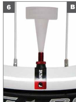
B. Sealant bottles often come with a funnel style cone cap that can be used if you do not have an injector.
