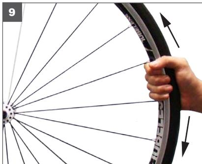
9. Once the beads are seated and the tire is holding air with sealant inside, shake and rotate the wheel to evenly spread the sealant until any small air leaks are sealed. Shake / rotate in many directions.
