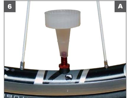
A. Inject the sealant using the funnel style cap or tube that came with the sealant.
