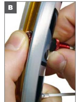
B. Firmly press base of valve into rim with your thumb then finger tighten knurled nut.
