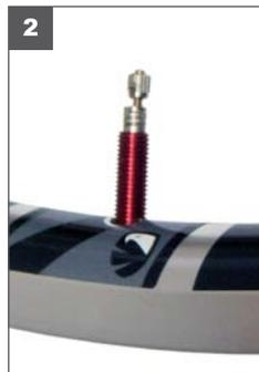
2. Insert red valve stem so the 2 rubber O-rings are touching the tape in the tire well.
