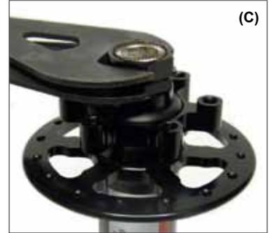
7. Grease the threads and install the new spacer with dust seal, install dust seal onto the adjusting nut and continue. A) Finger tighten the adjusting nut with the shoulder side facing the hub shell (B) Install the lock nut and finger tighten (C) Using two 19mm cone wrenches, remove all play on adjusting nut, then back off one half rotation, 180 degrees.
