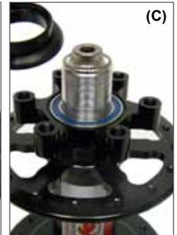
C. Remove spacer with attached dust seal.
