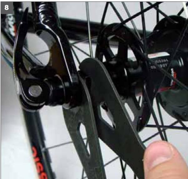
8. Place the wheel in the frame and clamp down quick release. Hold the adjusting nut in place with a 19mm cone wrench, still one half rotation loose from Step 7, tighten the lock nut against the adjusting nut. Once the lock nut is tight, check for the desired adjustment by wiggling the tire at the rim to feel for “slightly more than no play.” If the adjustment is not correct continue to Step 9.
