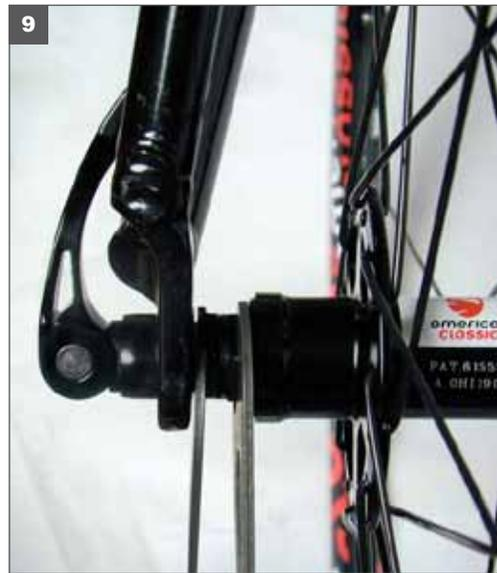
15. Hold the adjusting nut in place and loosen the lock nut. Slightly tighten or loosen the adjusting nut and hold in place. With the adjusting nut in place, tighten down the lock nut. Wiggle rim. Repeat Step 9 until the desired adjustment is achieved. Make sure the lock nut is tightened down when finished.
