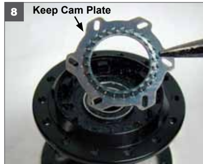
8. Remove cam plate. IMPORTANT: Keep cam plate for re-installation in Step 11.
