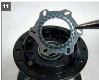
11. With a thin layer of clean grease coating the hub shell, re-install the cam plate. Refer to the picture for the correct orientation. Do not put the cam plate in upside down.
