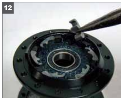
12. With a thin layer of clean grease coating the top of the cam plate, install all 6 pawls. Once completed, the pawls should freely engage in unison with the cam plate.
