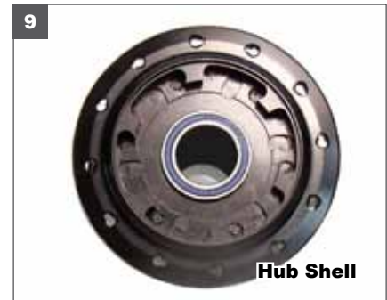
9. Clean out the hub shell for inspection and new grease.
