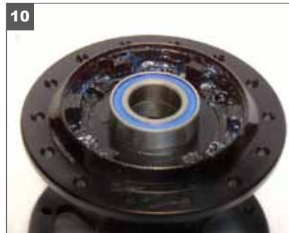
10. Bearing Installation: Position a new bearing onto the hub shell. Place old bearing on top of new bearing.
