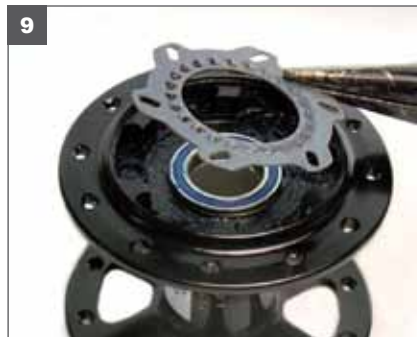
9. With a thin layer of clean grease coating the hub shell, install the cam plate. Refer to the picture for the correct orientation. Do not put the cam plate in upside down.
