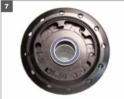
7. Clean hub shell for inspection and new grease.
